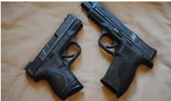
*You can see the textured grip surfaces on these guns. Both have been stippled to increase the friction between the hand and the grip. Beware of over stippling a carry gun though, as it will tear your cloths and skin up.*
